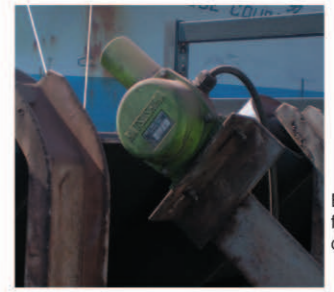
Belt Sway Switch for belt misalignment detection
