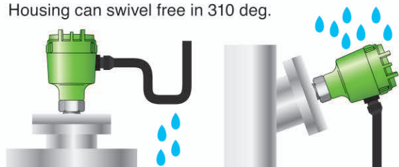
Prevent water intrusion by warping wiring cable
